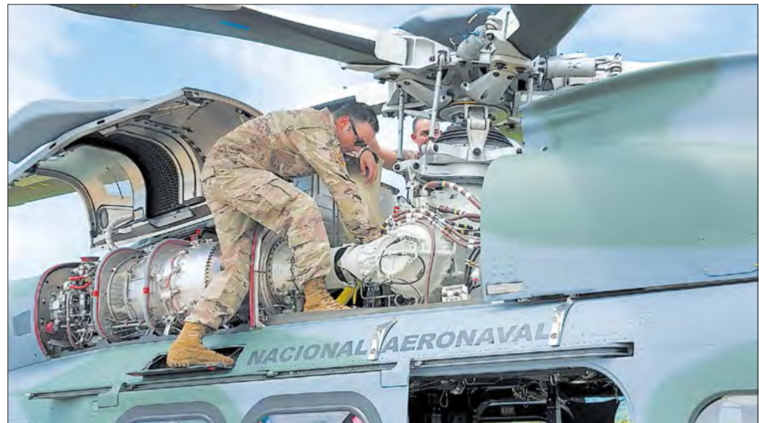
Master Sgt. Raphael Romero, 571st Mobility Support Advisory Squadron aircraft maintenance senior air advisor, performs a post-flight inspection on an Augusta Westland AW-139 helicopter engine along with the National Air and Naval Service of Panama flying crew chief at Nicanor Air Base, Panama. Air advisors assess, train, advise and assist U.S. Southern Command lines of effort of strengthening partnerships and countering threats from transnational criminal organizations.
